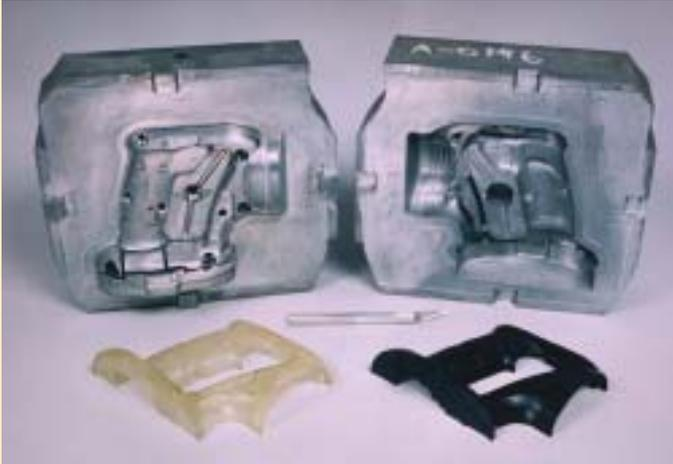
Thermoplastic hand tool prototype with SLA master and cast kirksite cavity.
