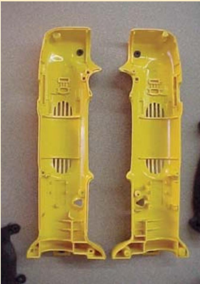
Prototype hand tool clam shell design.
