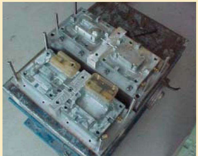
Cast kirksite cavity set for two parts molded together with SLA masters.
